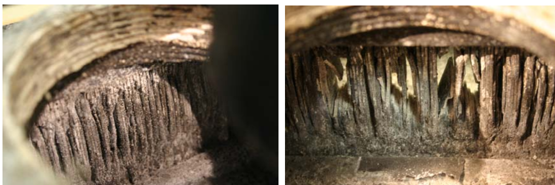
Figure 10. Flame arrester plate corrosion (inside)
