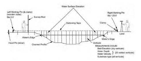
Figure 3. Illustration of Survey Technique and Data Collection at Each Study Site<sup>74</sup>
