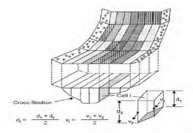
Figure 6. The Cross-Sectional Stream Profile as Broken Down in the IFIM/PHABSIM Method<sup>104</sup>
