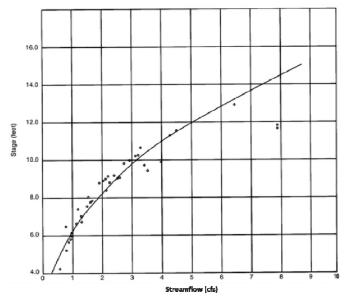
Figure 5. Example Rating Curve<sup>98</sup>
