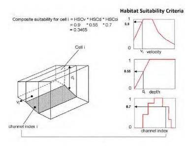
Figure 10. Example of a Water Cell Within a Stream Along with Representative HSC Criteria<sup>123</sup>
