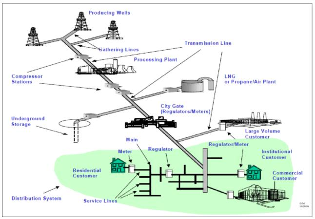
Figure 6. Schematic of the Natural Gas Delivery Pipeline Infrastructure. Generally, the distribution system entails the mains, service lines, and meter.
